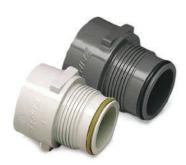
Rain Bird NPT-ACME or BSP-ACME side of the adapter. Just screw the adapter into the inlet on the ACME case, and then screw the rotor with the adapter onto the NPT or BSP swing joint until it is snug.
