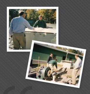
This first test was to determine that air would move easily through the soil mix of a USGA green and also that the pressure blower was capable of providing enough air.
