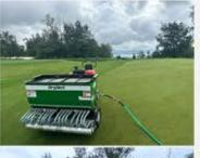
Centaur Asia Pacific recently conducted its first demonstration of the DryJect system in Hong Kong. The demo, held on a golf green, showed Profile Products being injected into the rootzone at a depth of 5 inches using a 3 x 3-inch grid spacing.
