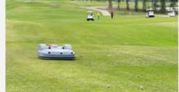
The Course Superintendent manages the mower through a web-based application accessible by phone, tablet, or computer. This allows for full control of mowing schedules and performance without the need for manual supervision. Since the rough at Hole 7 has been added to the same mower and plans are in place to expand the mower's working area across more sections of the course.
